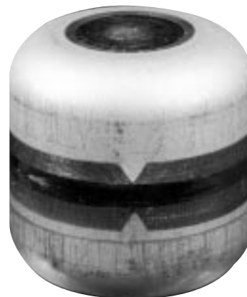
Figure 3. Photo of the GPHS iridium-clad capsule showing the equatorial tungsten arc weld and the iridium frit-vent at the pole, which releases helium from the alpha decay of plutonium. GPHS capsules are normally shipped to the Mound Facility for assembly into RTGs. The Cassini spacecraft employs 216 of these heat sources to provide thermal power for the three RTGs on the orbiter.
