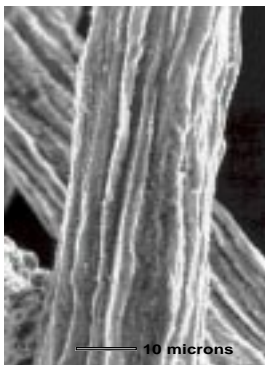
Figure 1. Scanning electron micrograph of extruded stainless steel matrix material. Results of experiments show that maximum separation effectiveness is obtained when the matrix fiber diameter approaches the diameter of the particles to be captured.
