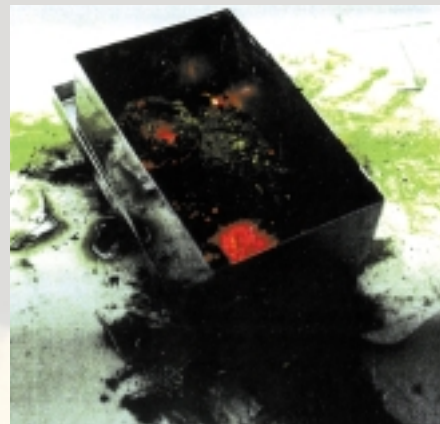
These glowing embers are small pieces of plutonium metal burning spontaneously in air under static conditions.
