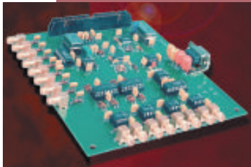
A SPECTRA circuit board. Input leads are attached from the eight transmitting ports on the left to the part and output leads are attached from the part to the eight receiving ports at the front of the board.
