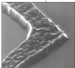
A highly magnified image of one of the aluminum metal lines towering above the flat silicon substrate after treatment with SCORR.
