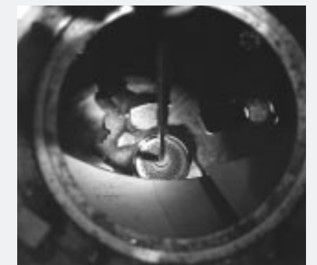
The last bit of extract containing the unstable germanium is drawn out from the gallium tank. The extract appears as a silvery pool floating on top of the duller, liquid gallium metal.
