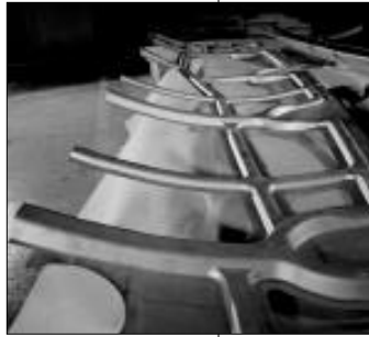
An aircraft engine’s nacelle waffle can be manufactured without costly trial and error, thanks to the Predictive Code for Superplastic Forming.
