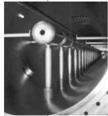
A view of the interior of the second stage of the Los Alamos accelerator, the drift-tube linac, where particles are accelerated to 80,000 miles per second (43 percent of the speed of light).
