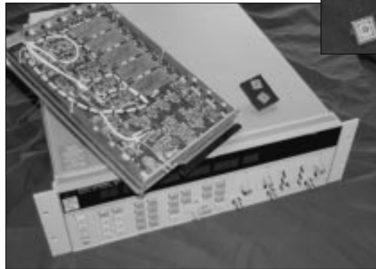
The top photo shows two of the Los Alamos integrated circuits. It takes at least two chips to make a time-interval meter. In the bottom photo, the chips and a circuit board from a previous-generation Los Alamos meter rest atop a time-interval meter sold by Hewlett-Packard.
