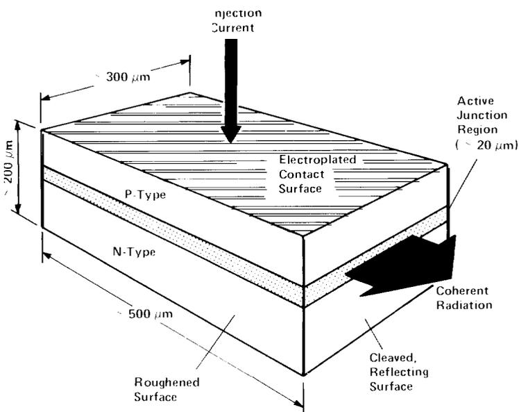
*Simplified diagram of a semiconductor diode laser. These tunable lasers have become the workhorses for molecular spectroscopy because of their broad coverage of the infrared region in which rotational-vibrational transitions occur.*
