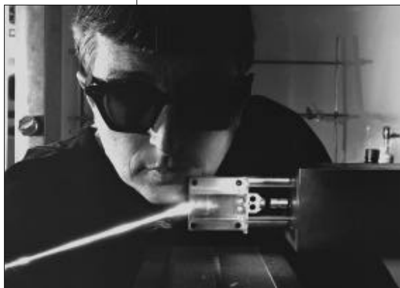
↑ Los Alamos researcher Gary Laabs aligns a laser to produce a speckle pattern of light on a block of high explosives.
