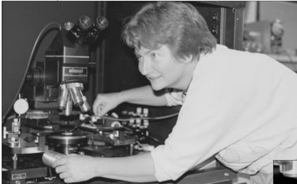
↑ Researcher Maureen Cafferty performs a quality control step on a new multi-chip module. Inset: The needle monitors voltages injected into the module.
