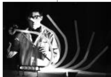
A researcher demonstrates the flexibility of a bendable heat pipe.
