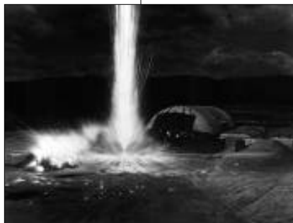
A dynamic test at the PHERMEX facility of a weapon design using conventional explosives but mockup fissile material. Another PHERMEX test is pictured on Page 24.
