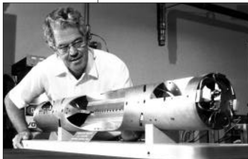
Scientist Ed Knapp with a cutaway model of the Radio Frequency Quadrupole.
