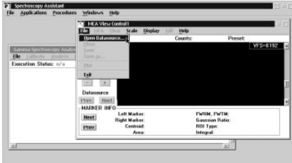
Figure 3. Window for opening a Datasource from within “MCA View Control.”
