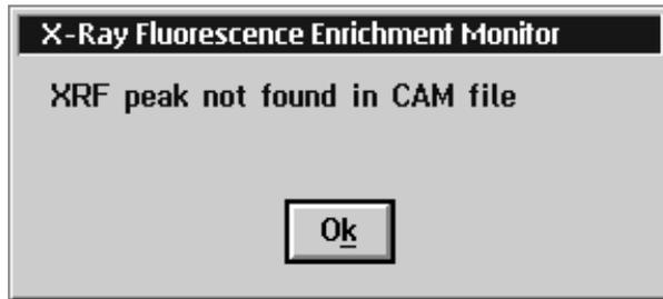
Figure 43. Message box indicating that no 98.4-keV x-ray fluorescence peak was found in the spectrum.
