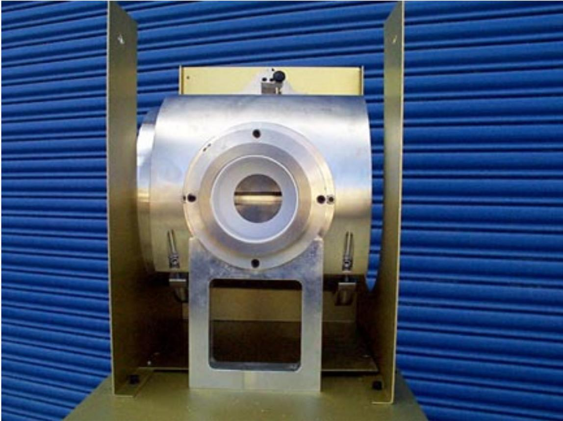
Figure 61. The detector collimator must be in the parallel, or horizontal, position. This is the only orientation of the detector collimator that will be needed initially. A direct deposit subtraction to the data is made, eliminating the need for the two-geometry technique. If the deposits change significantly during this verification exercise, then either the two-geometry technique will have to be used or the deposit will have to be remeasured.
