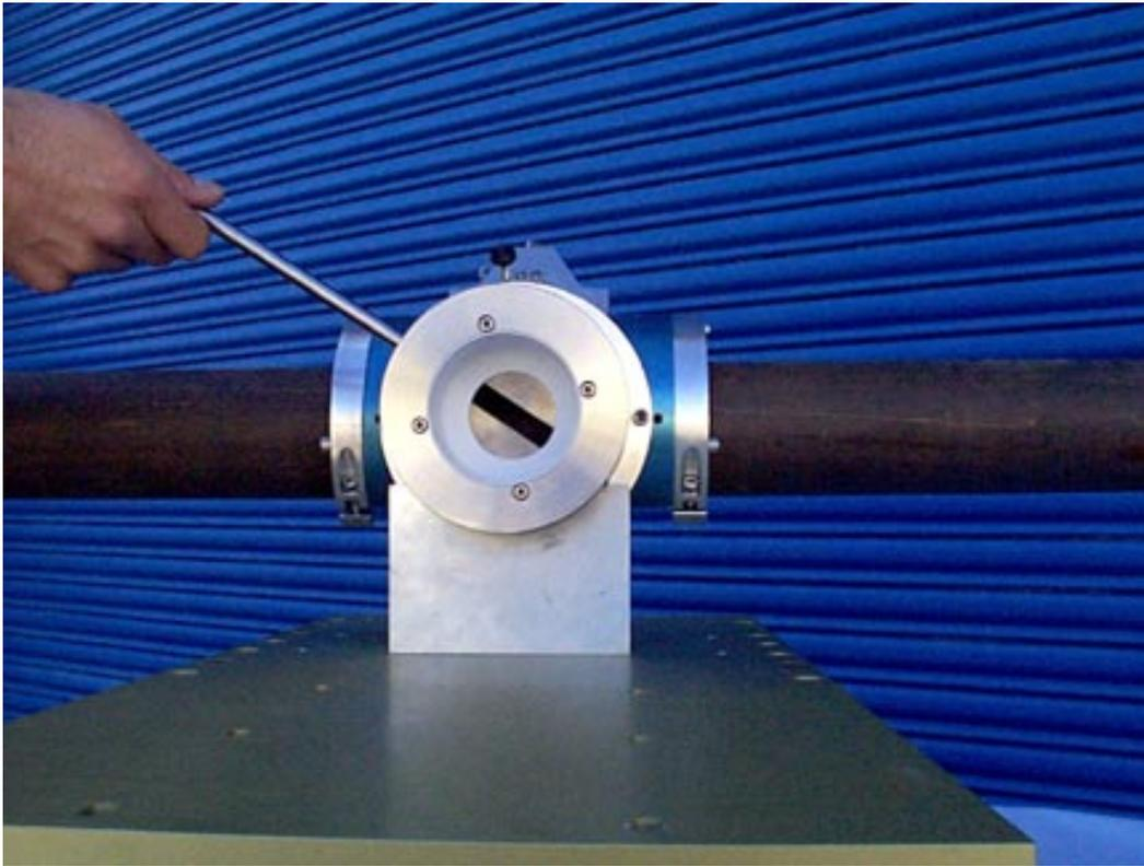
Figure 56. If the two-geometry technique is needed in the future, a special tool is supplied to ease rotating the detector collimator slit from the “parallel” position to the “perpendicular” position.
