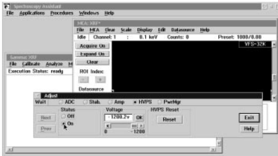
Figure 7. The “Adjust” window. Notice that the HVPS button is selected, the voltage is set to  $-1200.2$  V, and the “On” button is selected.
