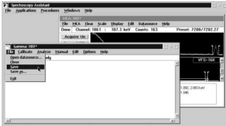
*Figure 22. Window showing the use of “Save” to save the new energy calibration.*
