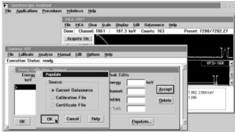
Figure 18. The “Populate” window, showing selection of the “Current Datasource” button and then the “OK” button.
