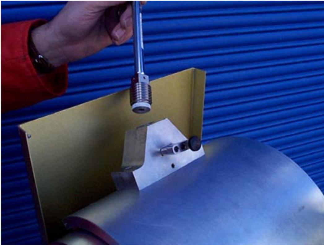
Figure 63. The XRF source is located at the end of the threaded tungsten source plug, behind the aluminum retainer cap.
