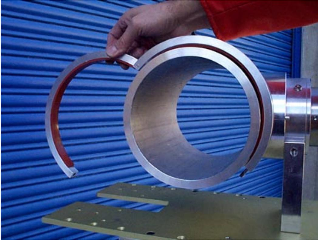
Figure 58. The collimator for the 8-in. (20.32-cm) header pipe is placed in position around the header pipe. The clamps, one on each edge of the collimator, need to be opened for the collimator to initially fit over the pipe. The collimator is already attached to the “saddle” and the base plate.
