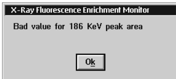
*Figure 42. Message box indicating that the 185.7-keV  $^{235}\text{U}$  peak area is negative.*
