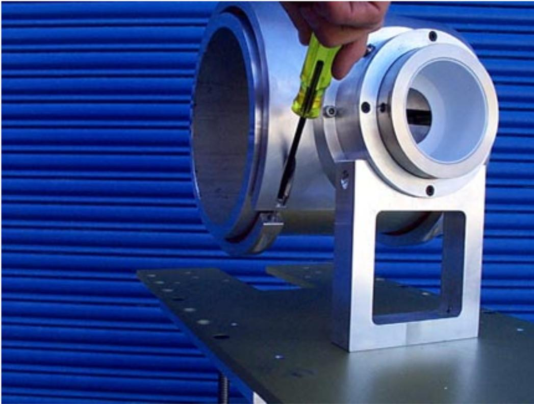
Figure 59. Use an Allen wrench to initially tighten both clamps around the header pipe.
