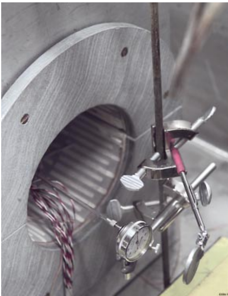
Fig 4 – Close up of dilatometry set up. Note quartz rod attached to dial indicator.
