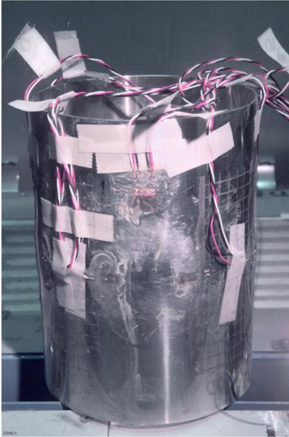
Fig 15 – Cylinder after six thermal cycles. Note plastic deformation around center of cylinder. Cylinder is 6" in length.
