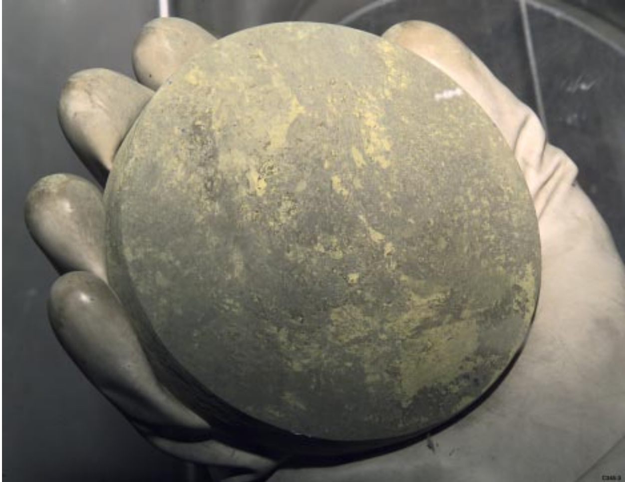
Fig 16 – Pu ingot after six thermal cycles showing moderate surface oxidation.
