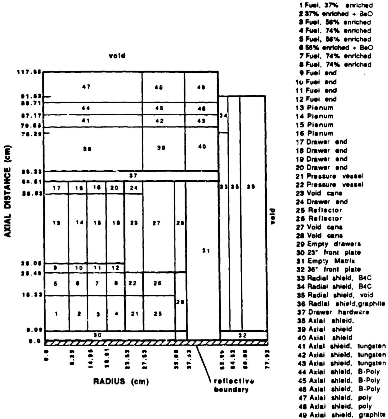
Fig. 9 r,z Calculational Model
