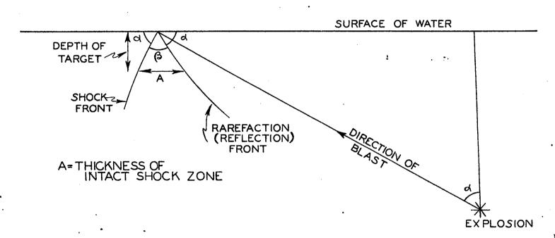
FIGURE 2. GEOMETRY OF SHOCK WAVE REFLECTION ILLUSTRATING REQUIRED DEPTH OF EXPLOSION
