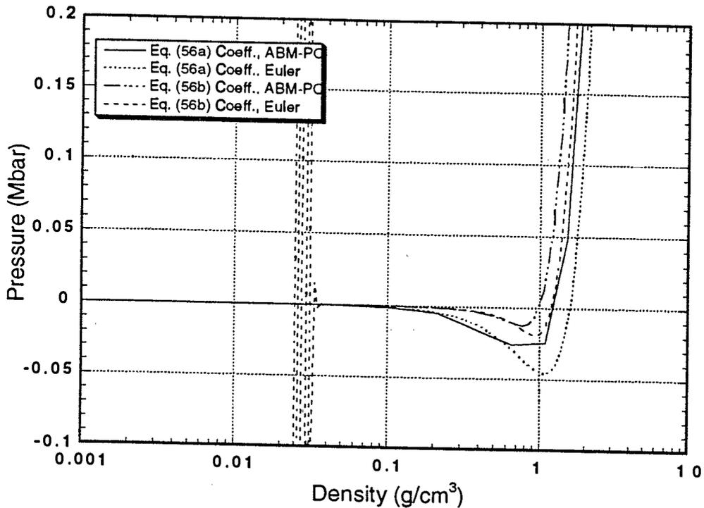
Fig. 14. Pressure ( $P$ ) as a function of density ( $\rho$ ) along an isentrope through 10 Mbar on the Hugoniot for a Mie-Grüneisen EOS for Al.
