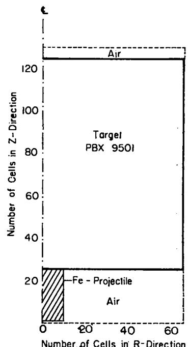
Fig. 3. Typical computer model for an impinging cylindrical projectile.
