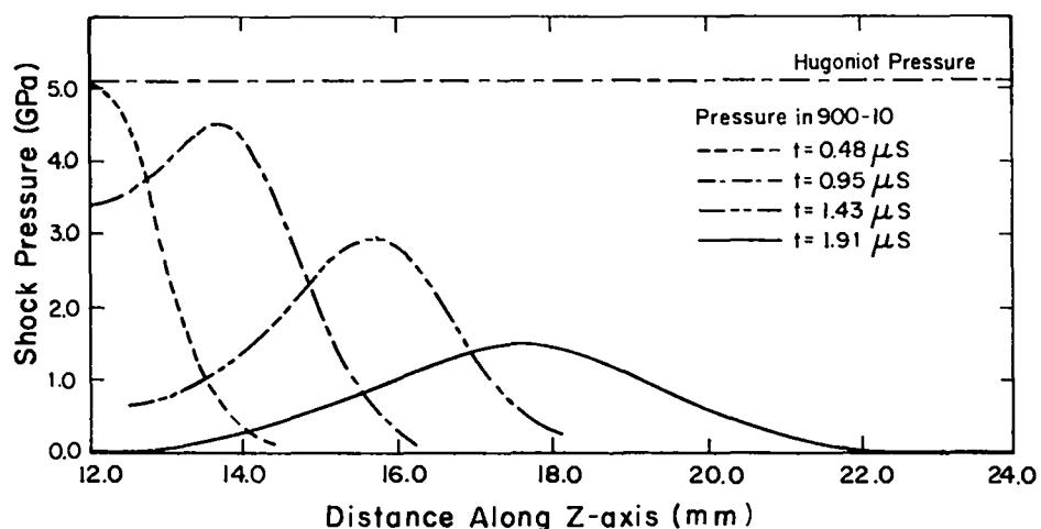
Fig. 4. Calculated pressure along centerline for 7.62-mm-diam cylinder impact on 900-10 at 845 m/s at various times after impact.
