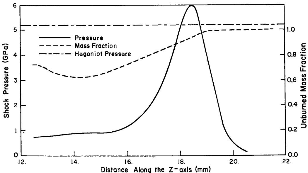
Fig. 6. Calculated pressure and unburned mass fraction for 7.62-mm-diam cylinder impact on PBX 9501 at 845 m/s, 1.91  $\mu$ s after impact.
