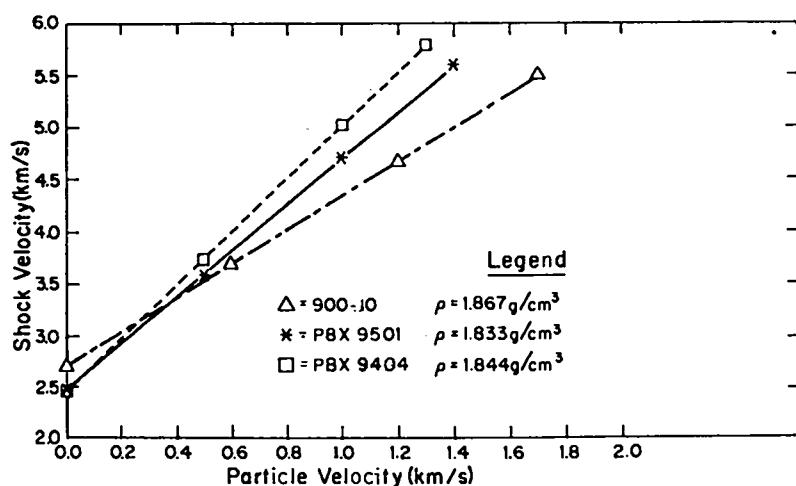
Fig. 2. Shock-particle velocity relation for 900-10, PBX 9501, and PBX 9404.
