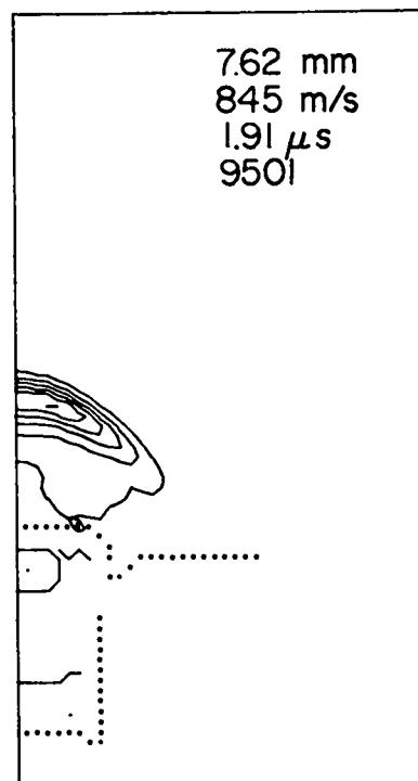
Fig. 7. Calculated isobars in PBX 9501 at 1.91  $\mu$ s after impact by 7.62-mm-diam cylinder at 845 m/s.
