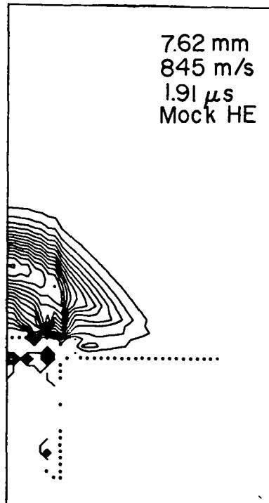
Fig. 5. Calculated isobars in 900-10 at 1.91  $\mu$ s after impact by 7.62-mm-diam cylinder at 845 m/s.
