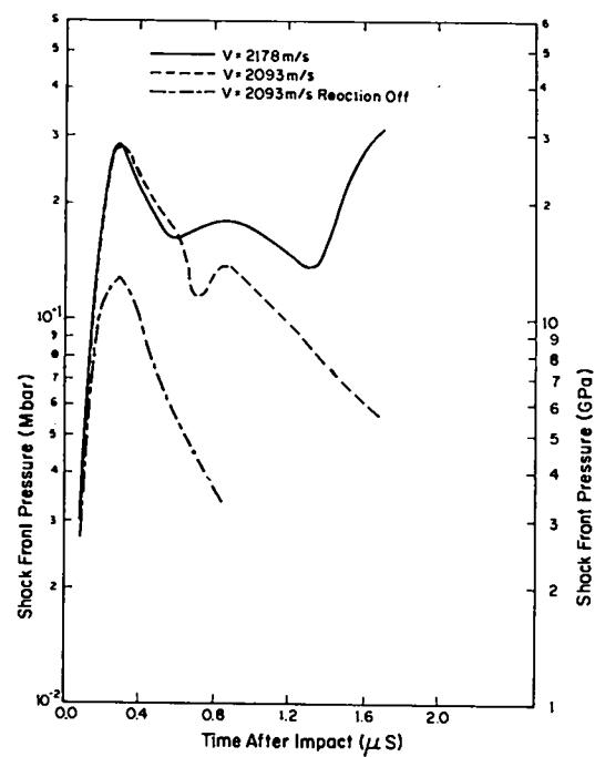
Fig. 10. Shock front pressure versus time for impact by 3.35-mm-diam cylinder.
