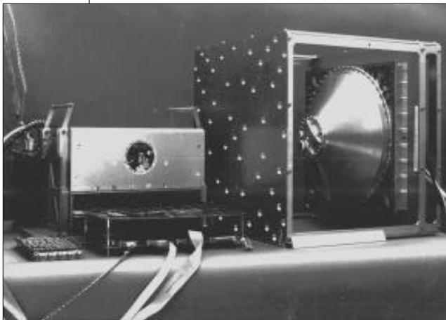
MOXE's development included initial delivery in early 1992 of a model that was subjected to thermal, vibrational, and static load testing. That was followed by an engineering model delivered to Russia in November 1993, which passed a series of complicated acceptance tests. The MOXE team is now
