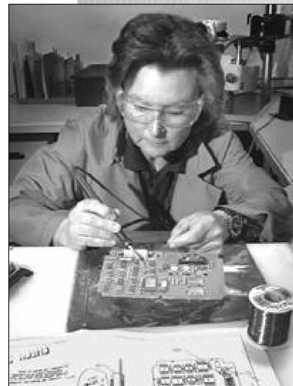
Irma Gonzales of Space Engineering (NIS-4) "stuffs" a printed circuit board with electronic components. The board, and a dozen or more like it, will be part of the instrument package on board a space mission. Photo by Fred Rick
