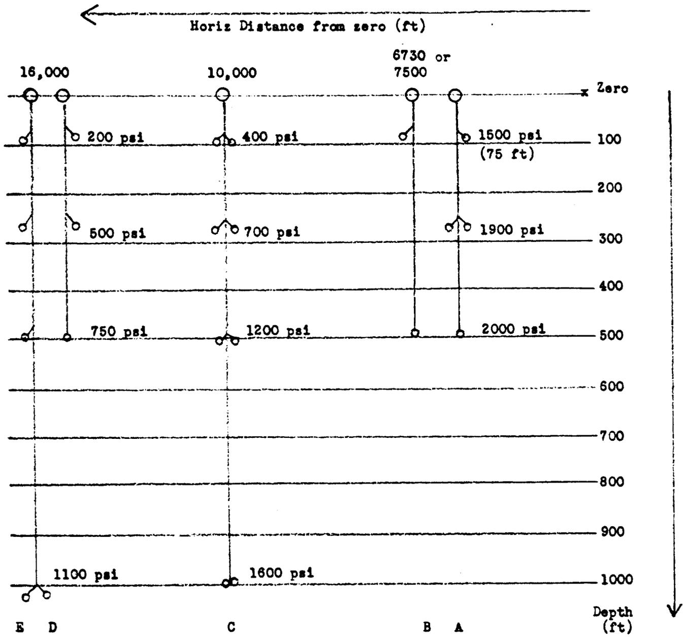
Instrument Line "A" is a 4-channel NOL system; "B", a Hastings system; "C" is an 8-channel Wiancko system.
