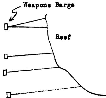
It is thought that a 1-1/2" chain should be sufficient to go from the moorings to the water. Then a 1/2" wire cable with breaking strength of 28,000 lbs will be adequate from the cable to the buoys. A deep sea moor will be put down to a 2800 lb anchor with a 1-1/2" chain leader. The instrument cans will be fastened to this system.
