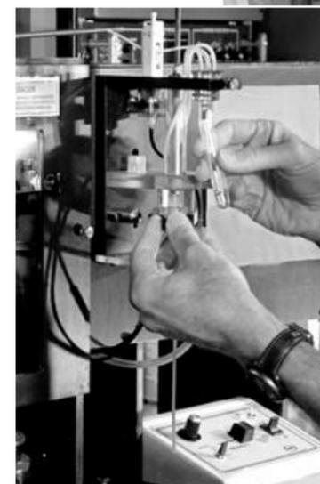
Left: A sample is carefully placed into a holder from where its content can be fed through the flow chamber and analyzed. The Lab's flow cytometers can determine the size, shape and functions of thousands of cells in seconds, and they are used for up to a dozen different experiments a week.
