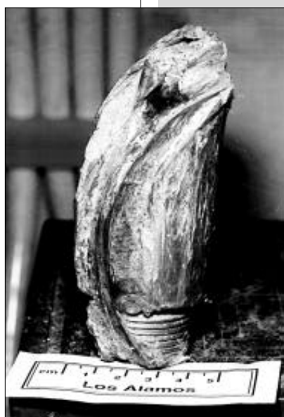
↑ A damaged americium-beryllium neutron source recovered from a private company by Los Alamos.
