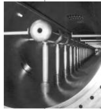
A view of the interior of the second stage of the Los Alamos accelerator, the drift-tube linac, where particles are accelerated to 80,000 miles per second (43 percent of the speed of light).
