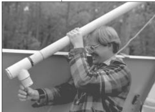
↑ Newman empties a runoff sample from the collection pipe into a vial.
