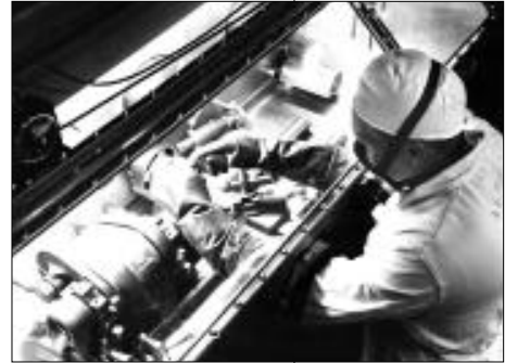
A worker handles special nuclear materials in a glove box at the Laboratory's plutonium processing facility.
