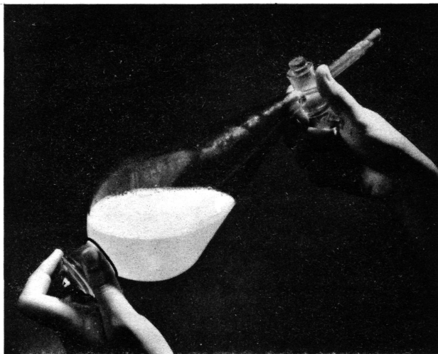
FIG. 13a. Proper method for holding a separatory funnel.
