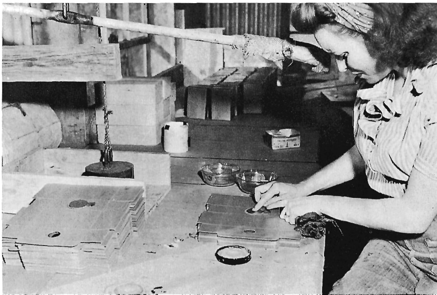
Fig. 10.6. — Glueing on the Tear Tab (Depression of the lever raises a weight for insertion of the freshly glued cartons.)
