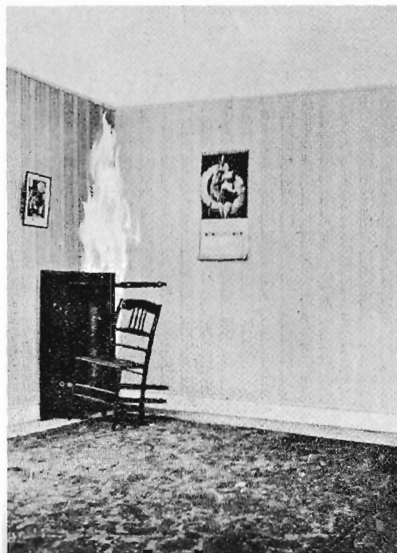
Fig. 19.11. — Pocket Incendiary operated in the space between a wall and the top of a turned-over table
